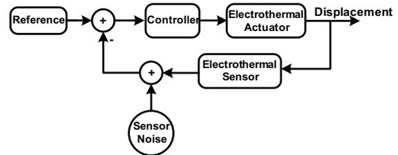
Fig. 1. Micro-actuator feedback loop block diagram.
