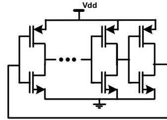
Fig. 8. Ring oscillator using digital inverter chain.
