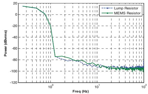
Fig. 14. Noise power spectrum of demodulated output.
