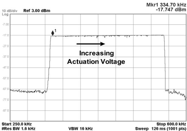
Fig. 13. Ring oscillator frequency versus actuation voltage.
