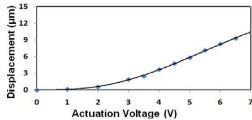
Fig. 5. Nonlinearity of actuator transfer function.
