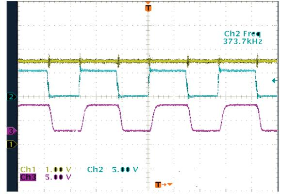
Fig. 11. Tracking VCO outputs and FM demodulated output: Ch2 (VCO1 output), Ch3 (VCO2 output), and Ch1 (demodulated output).
