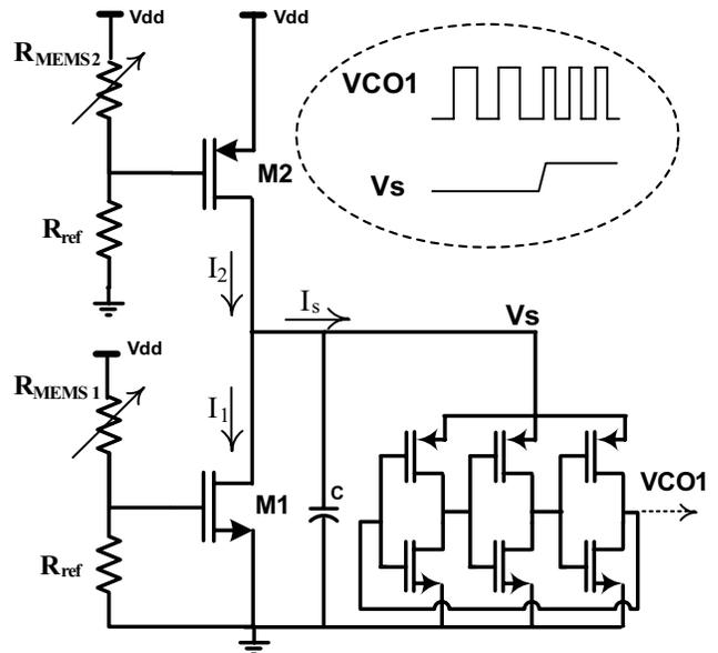
Fig. 10. Circuit designed for VCO1 in proposed system.
