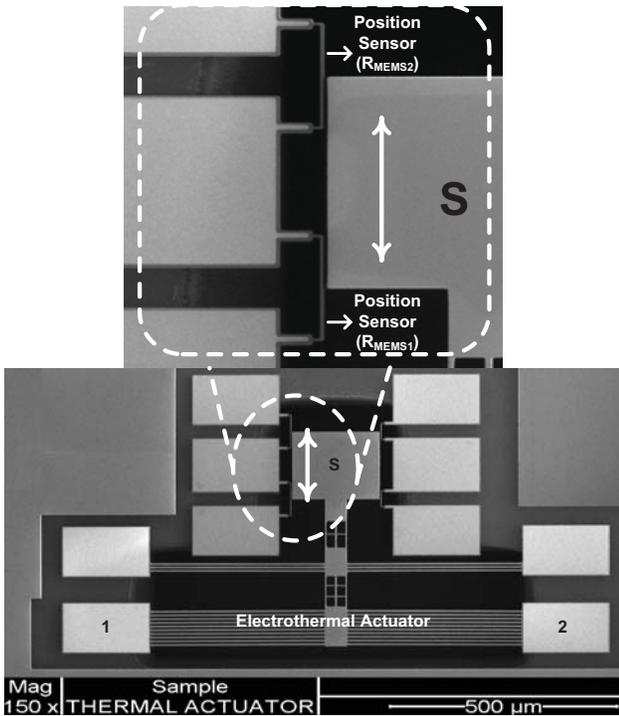
Fig. 2. MEMS-based thermal sensor and thermal actuator.
