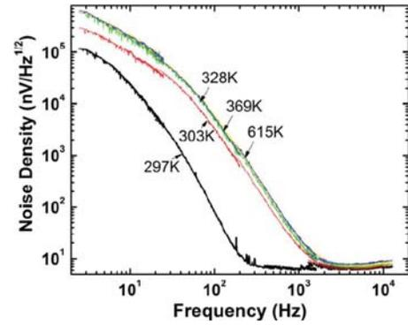
Fig. 3. Doped silicon cantilever noise power density [13].
